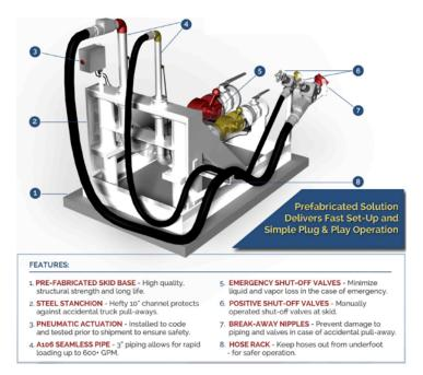
Liquid Transfer Skids Loading and Unloading solutions with customizable options to include liquid pump, compressor, metering and other instrumentation for all skids. Prefabricated to industry standard and tested inhouse to reduce installation time. Skid packages include all of the equipment and installation hardware to allow immediate use, ease of options and built by our industry leading design and manufacturing teams.
