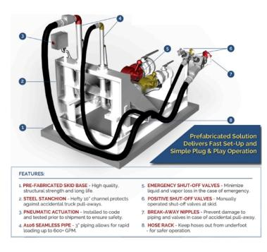
Liquid Transfer Skids Loading and Unloading solutions with customizable options to include liquid pump, compressor, metering and other instrumentation for all skids. Prefabricated to industry standard and tested inhouse to reduce installation time. Skid packages include all of the equipment and installation hardware to allow immediate use, ease of options and built by our industry leading design and manufacturing teams. Prices start at:
